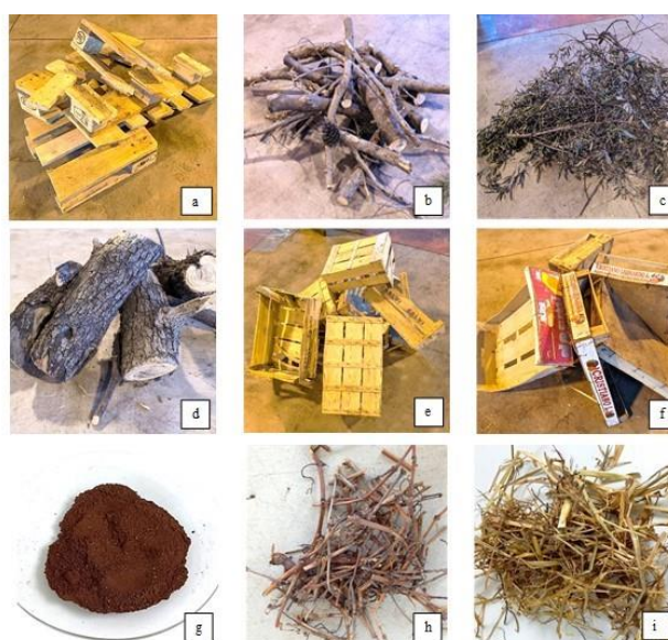
Fig. 4 - Biomass samples: a) pallets, b) pine logs, c) olive twigs, d) olive trunks, e) wooden crates, f) crates with particleboard elements, g) olive pomace, h) vine shoots, i) wheat straw
